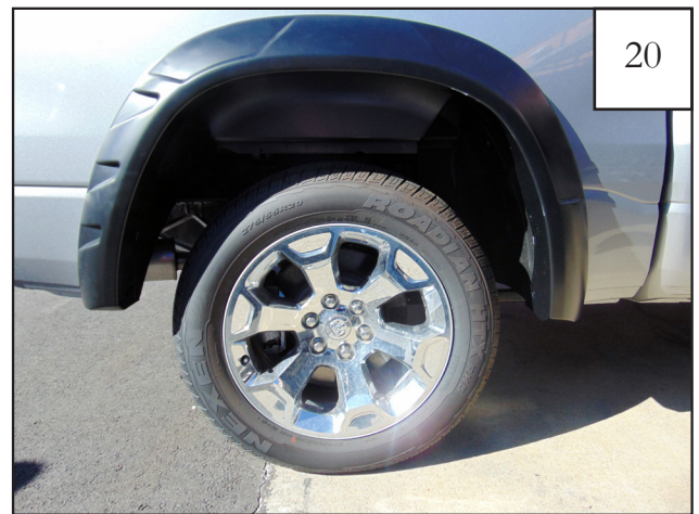
Completed rear flare installation.
